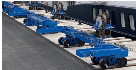
Figure 2 A rail based self-propelled transfer system.
